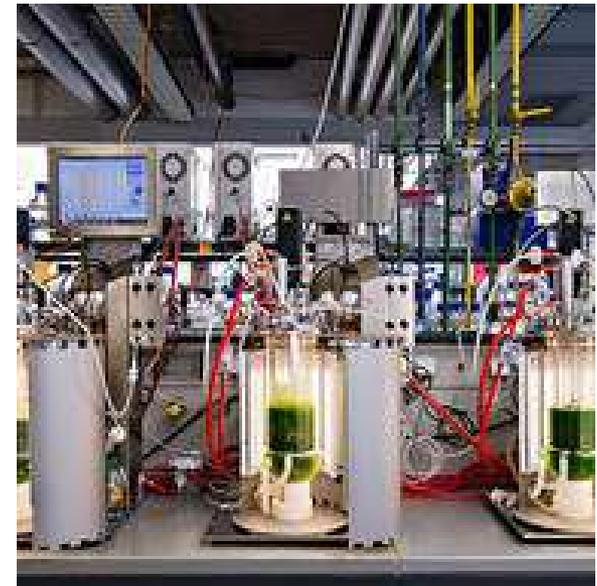
Laboratory bench with LED-bioreactors –
